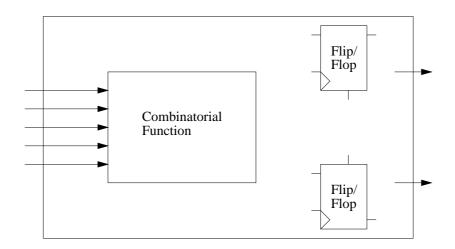
Figure 5: Configurable Logic Block.
