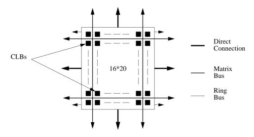
Figure 7: Interconnection Scheme of one LCA.
