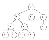
$$\begin{split} \text{Let } \mathcal{A} &= (\{a, I\}, \{q_a, q_c, q_I\}, \{q_a\}, \Delta) \text{ where} \\ \Delta &= \left\{ \begin{array}{ll} a \left[q_a^*. q_I^*. (q_c \mid \epsilon)\right] & \rightarrow q_a \\ c \left[q_I\right] & \rightarrow q_c \\ I \left[\epsilon\right] & \rightarrow q_I \end{array} \right. \text{ Special rule for leaves} \end{split}$$
