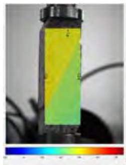
X displacement of a sample by DIC
