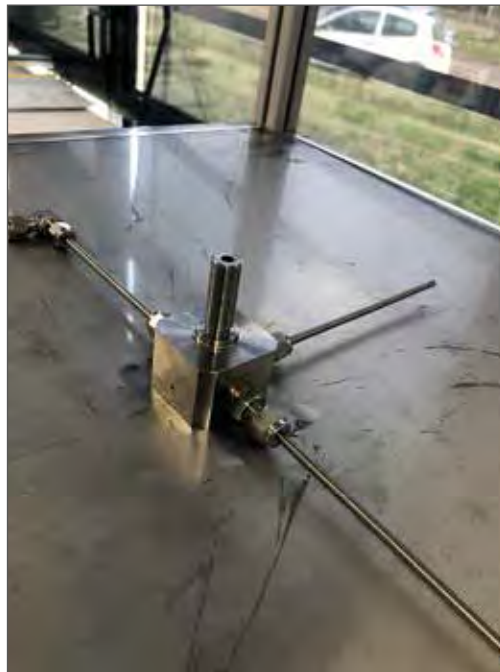
Igniter mounted on the test bench
