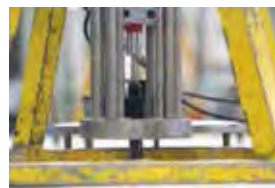
Displacement measuring during a pull-out test
