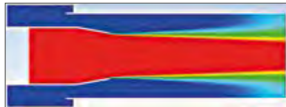
CFD simulation of the flare before optimization
