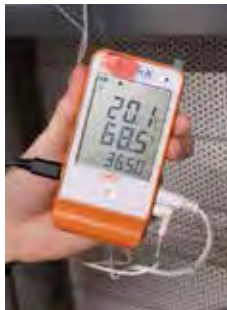
Hygrothermal device (displayed: temperature/relative humidity/number of measures logged)
