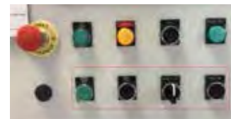
Real dashboard on the real Solujet machine
