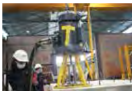
Pull-out test with the hydraulic jack at the CSTB
