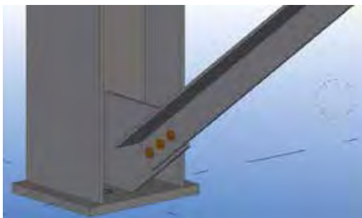
Drawing of the connection with angle calculated by the Excel sheet
