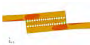
Numerical simulation of a modified lap-shear test
