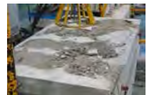
Resulting concrete slab after removal of cones
