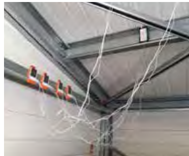
Hygrothermal device and dataloggers for heatflow sensors (for the roof in this case)
