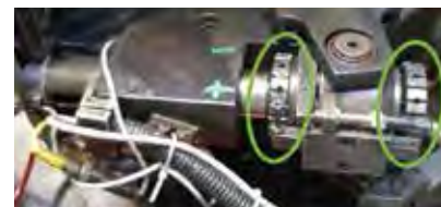
Adjustment wheels for press-fitting and crimping parameters
