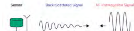
SAW sensor (source www.teansense.com )
