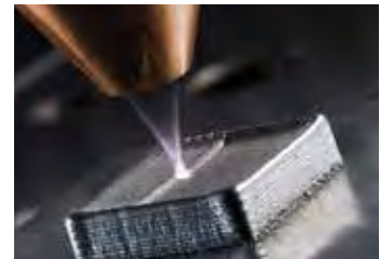
Plasma treatment with ICP Corial reactor
