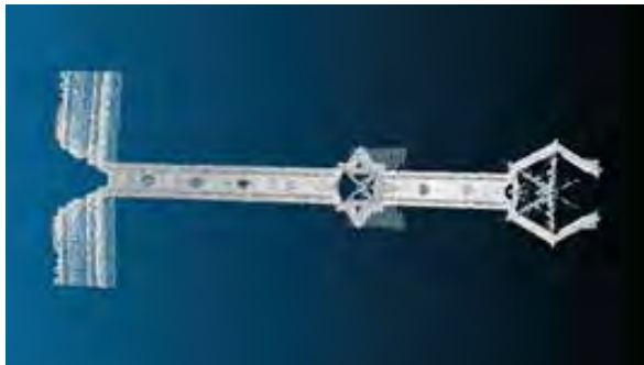
Flying buttress as a point cloud, view from above
