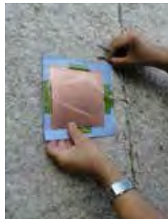
heatflow sensor placed on insulating material
