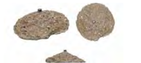
3D model of a concrete rupture cone obtained using photogrammetry
