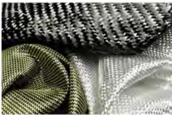
Aramid fibers (left), carbon fibers (upper), glass fibers (right)
