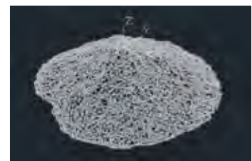
Autocad model of a concrete rupture cone
