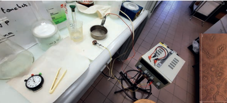
Material used during the electrolytic attack
