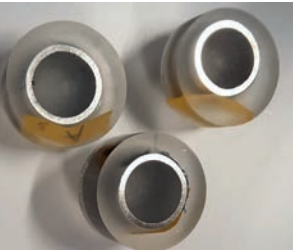
Duplex steels samples after sampling and coating
