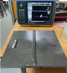
ultrasound testing of defect
