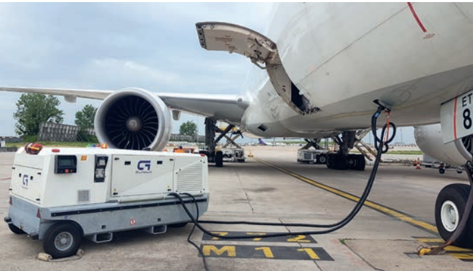
Ground power unit in operation
