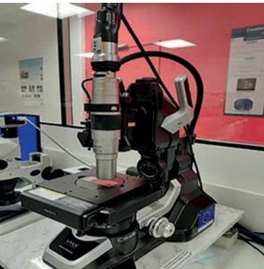
A sample on the numerical microscope being characterized in the clean room
