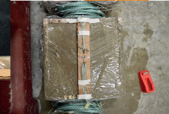
Concrete cube + thermocouples
