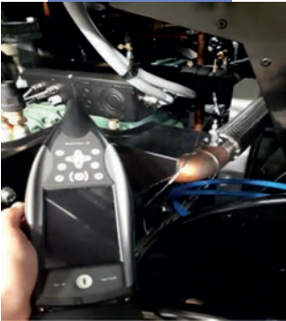
Vibration measurements on a refrigeration line
