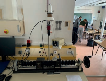
Traction machine of the practical image correlation
