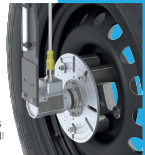
Speed sensor for the Coast Down
