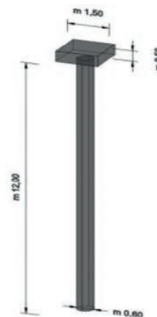
Rigid Inclusion Model and Dimension
