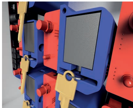
3D render of the Key block view : the key block board in red, with its button and LED. The key is held with a solenoid
