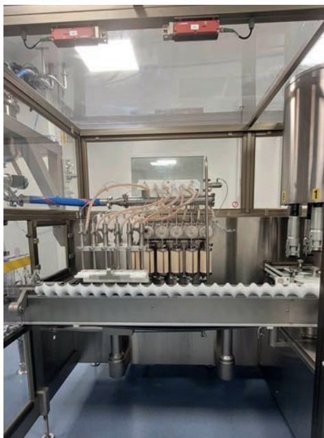
Bottle filling module for primary packaging
