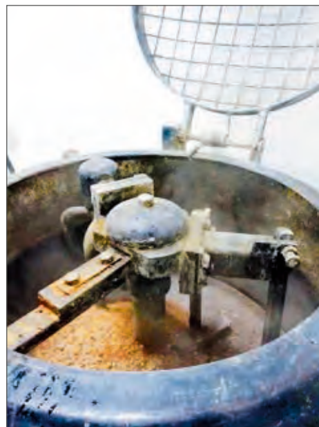
Production of concrete specimens by using the mixer
