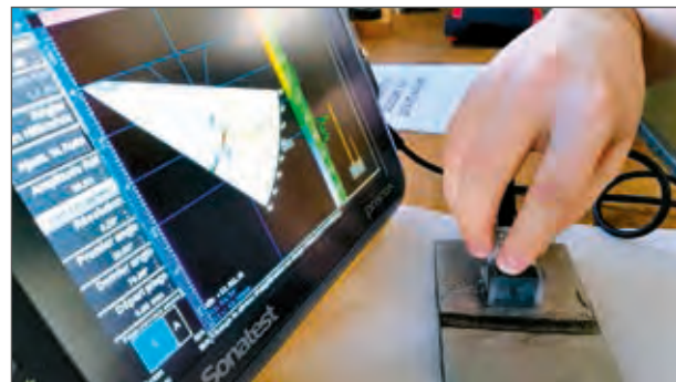
Ultrasonic inspection using the phased array probe
