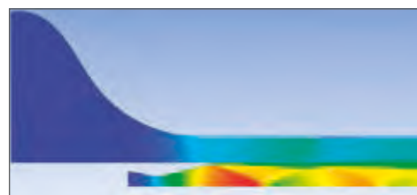
Contour of Mach number for the saturated-supersonic regime
