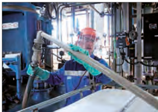
Pipe that allows products from outside the circuit to be loaded into the reactor
