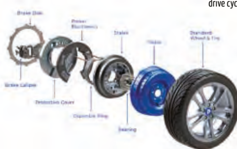
In-wheel motor technology (Protean Drive™)
