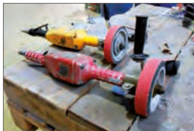
These tools will be attached to the mechanical arm and used to polish the tanks
