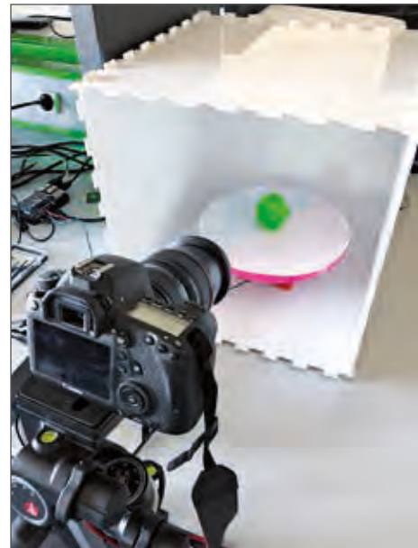
Complete acquisition system, with photo box and SLR camera
