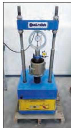
Californian Bearing Ratio (C.B.R) test
