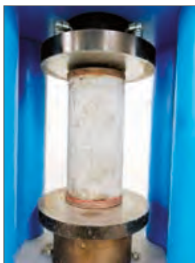
Compression test of a concrete sample to determine its strength
