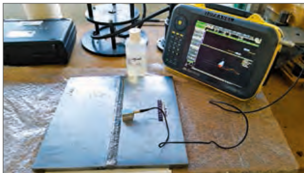
Ultrasonic inspection using the conventional probe
