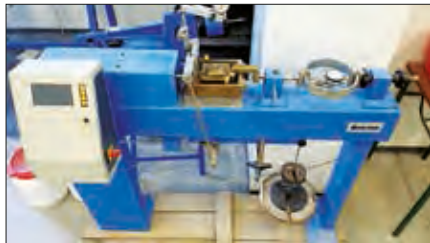
Shear test, Casagrande box
