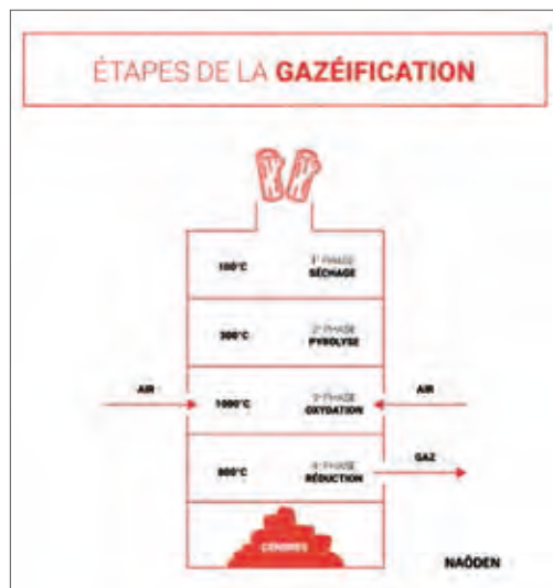
Steps in the gasification process
