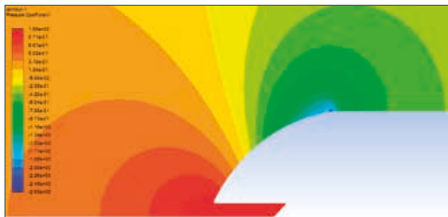
Pressure coefficient distribution on the front of the shuttle
