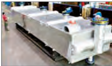
Brazed Aluminium Heat eXchanger (BAHX)
