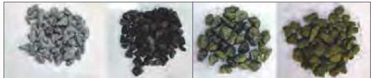
Natural gravel and coated gravel obtained after three different tests with different proportions of pigments and bitumen emulsion
