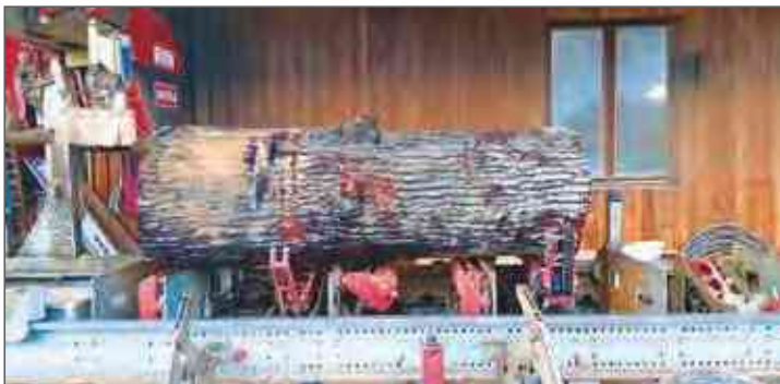
A Serra bandsaw mill at work
