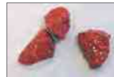
Aggregates coated with the resin/coloring paste mixture
