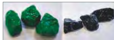
Aggregates coated with a coloring layer of acrylic paint and a protective layer of resin
