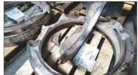
Example of granulation chain break
