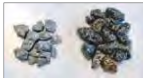
Natural gravel and coated gravel with uncolored resin
