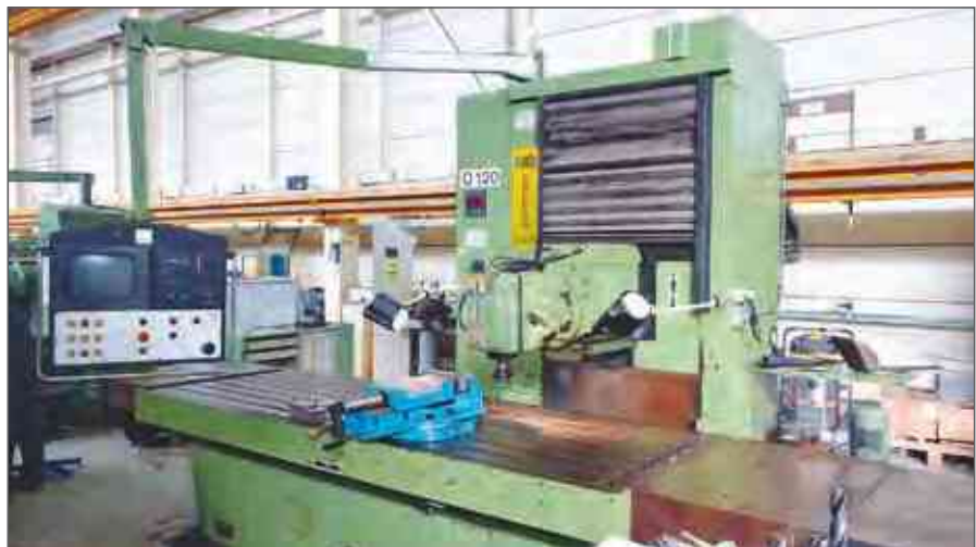
The 3-axis milling machine which requires an electrical retrofitting
