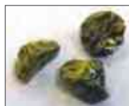
Aggregates coated with the resin/coloring powder mixture
