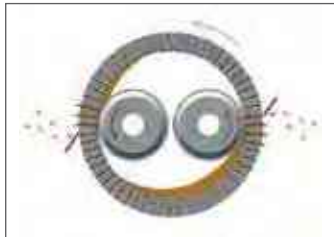
Function of a granulation chain with its rollers inside
