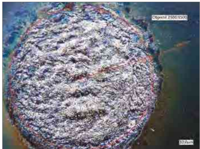
Observation of laser-induced damage on silicon
