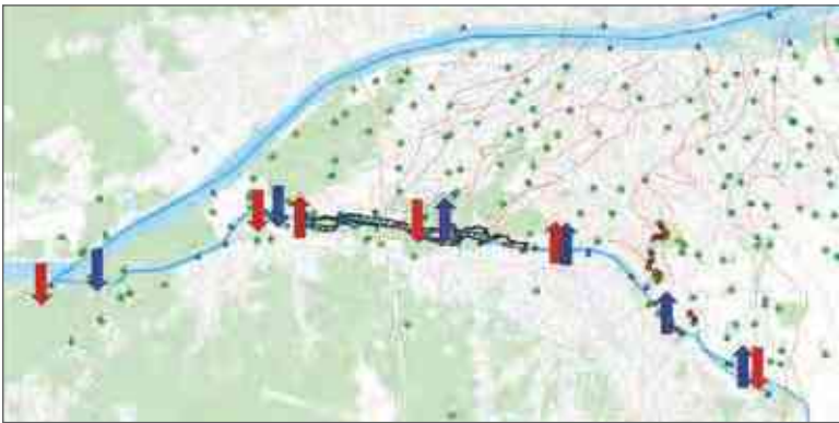
Simplified view of the GIS showing the direction of the exchanges between the ground water and the river
