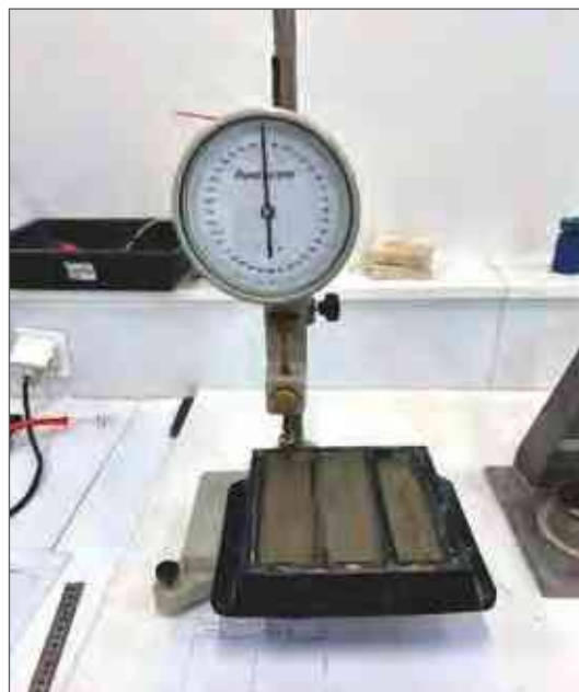
Fall cone test for consistency of mortars
