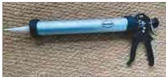
Manual gun for extrudability test of 3D-printing mortars
