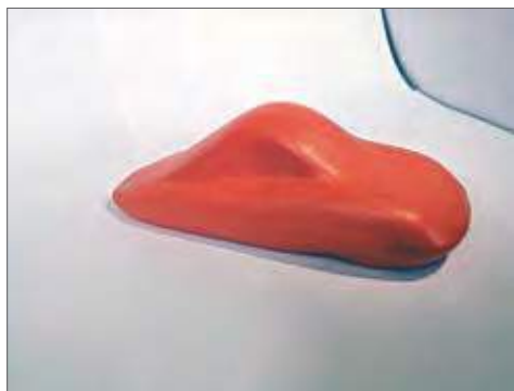
Small scale model of one of the vehicles made with polyurethane foam
