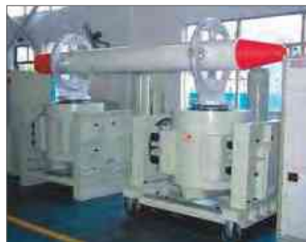
Example of fatigue damage test on a rocket (source: Crystal Instrument)
