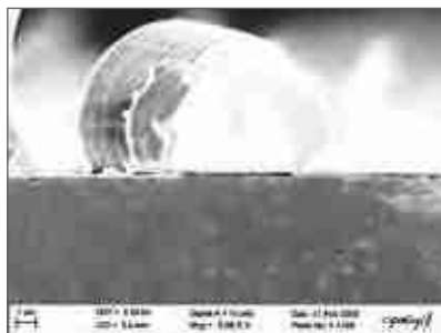
Failed deposition with delamination of the layer
